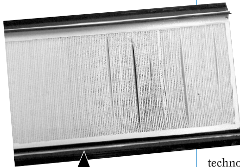
Constant freezing and thawing in a cold climate has caused the paper ERV core to separate and deteriorate.
