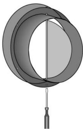
Push and turn with slotted screwdriver. Damper automatically locks when pressure is released.
