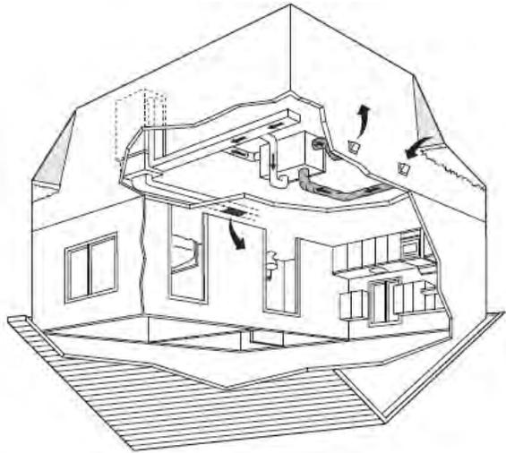
RACCORDS DIRECTS DU CIRCUIT DE DISTRIBUTION D'AIR DU VRE ET DU CIRCUIT D'AIR ÉVACUÉ À LA REPRISE D'AIR FROID DE LA FOURNAISE
