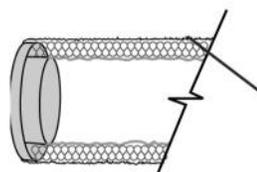
Insulated flexible ducting
