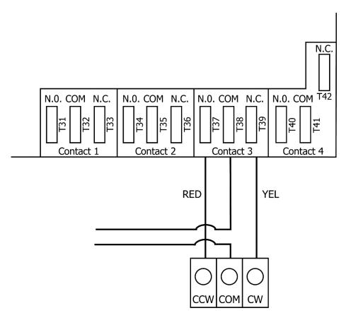
Switch T37 (red wire) and T39 (yellow wire) on the circuit board if you wish to reverse the "Supply Air from Outside" and "Defrost Air" ports. This illustration shows the factory configuration.
