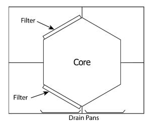
**Note:** When removing cores and filters, note their location and arrangement.
