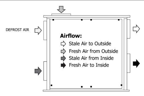
Sometimes installation is easier if the "Fresh Air from Outside" is ducted from the upper left side port (Defrost Air) instead of the top port. Changing the functionality of these two ports is easily accomplished by switching the red and yellow defrost motor wires at the circuit board: switch T37 and T39 on the circuit board.
