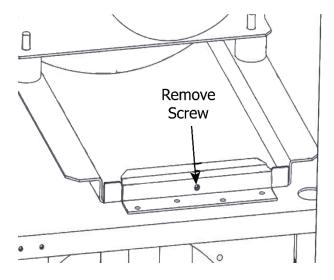
7. Remove the ground continuity screw from both the upper and lower blower pans securing them to the pan stops.
