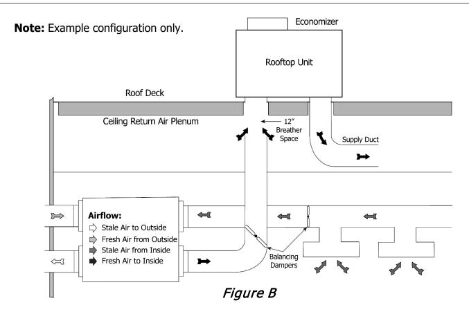
Many buildings have ceiling return air plenum as in Figure B. Fresh air from the HRV can be introduced directly into the ceiling space, but this should occur near the air handler's intake.
