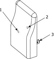
The 99-RX02 repeater should be installed at the halfway point between the 99-DET02 wireless timer and the main wall control if the timer is out of range. The LED will indicate the repeater's connection strength to the main wall control per the table below. Re-adjust the repeater's position as necessary.
