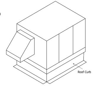
**Note:** Roof curb is one inch smaller than outside dimension of cabinet
