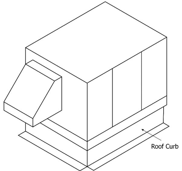
**Note:** Roof curb is one inch smaller than outside dimension of cabinet
