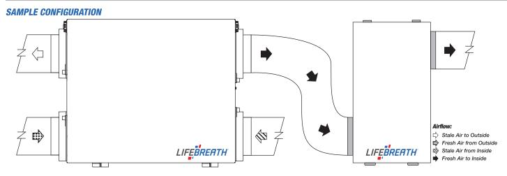
NOTE: Airflow may be reversed in warm climates (ie - fresh air from outside directly to the Lifebreath SCRUBBER, then to the HRV/ERV).
